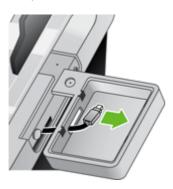
Install the hardware integration pocket on the product as shown by rotating the pocket into place, and then secure the pocket with the screw you removed in Step 2.
